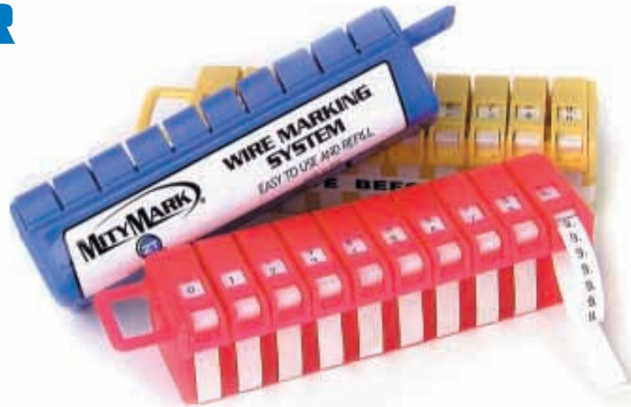
Simply pulling down on this liner feeds the marker from the dispenser and makes it ready for application. In addition to 0-9, legends A-Z and NEMA colors are available as stock items. Since the dispenser is refillable, replacement markers may be ordered by the roll or in boxes of 10.
