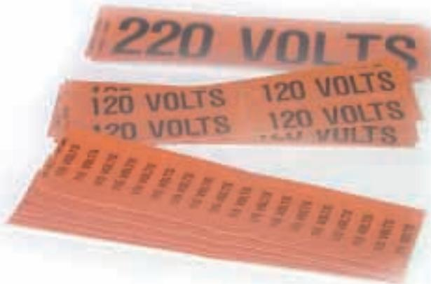
Ziptape® voltage markers are designed specifically to identify conduit, cable trays, load centers, busways, circuit breakers, switches, fuse boxes and other vital electrical equipment. There are three styles of markers, all on a 2.25" x 9" card. The marker is made of heavy gauge orange vinyl, and the adhesive is high tack acrylic. Voltage markers are packaged with 5 identical cards per polybag.
