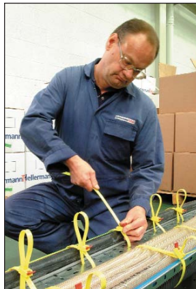
Temporarily bundling of unfinished parts or cables in an assembly line or a construction project.
