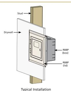
Flush mount in-wall housing. Standard color of lid is beige, and the standard color of the box is grey.
