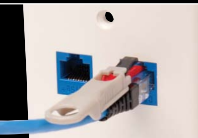
Remove lock with key to unplug connector
