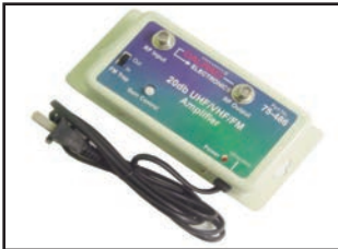
75-486 UHF/VHF/FM AMPLIFIER - 20dB Amplifier with adjustable gain control. 20dB amp. Switchable FM attenuation trap, ON-OFF indicator light. Frequency response of 5 to 900 MHz. Size: 1.47"(H) x 2.93"(W) x 5.65"(L).
