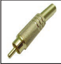
30-387 Gold 30-387-NK Nickel Heavy duty gold or nickel RCA Audio Plug for use on cable up to RG59 coax. Spring strain relief. .28" cable opening.
