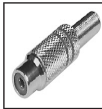
30-351 Red 30-353 White Gold plated RCA Audio & Video inline jack with color coded band, knurled barrel and strain relief. .21" cable opening.
