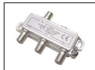
75-714-3 3-WAY 1GHZ DIGITAL SPLITTER 1GHz, 130dB splitter. Digital ready CATV splitters designed for hybrid distribution networks, voice-data, modem and digital converter applications. Fully water resistant. Soldered rear cover 130dB min, EMI-RFI shielding, DC blocked and IEEE-587 built-in 6kV surge protection at all ports. High performance components and circuitry. Anti-corrosion tin plated zinc-alloy, die cast housing. Mounting tabs with screws, cast-in ground block. Insertion loss 5.5-5.9dB max, isolation 35dB min, isolation 21dB min 40MHz-1GHz. Return loss 22dB min 15-40MHz.
