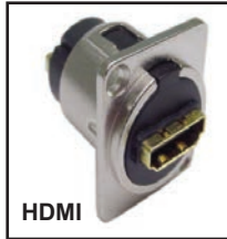
35-723 'D' Style panel mount HDMI female-female feed-thru. Gold plated contacts. Mounts in a .917" hole.
