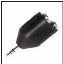
35-553G-HG High Grade 35-519G Gold version Shielded "Y", two 3.5 mm stereo jacks to single 3.5 mm stereo plug, gold.
