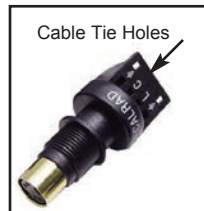
35-498K-S Solderless Keystone & Chassis Mount SVHS Jack. Easily mountable SHVS jack for either 1/2" chassis mount or keystone insert. Screw terminals provide a clean, solderless, connectorless backside termination. Includes cable tie for strain relief. Colored plastic washer available for enhanced visual ID (Part Number 30-288-Color).
