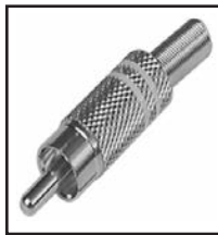
30-350 Red 30-352 White Gold plated RCA Audio & Video Plug with color coded band, knurled barrel and strain relief. .21" cable opening.
