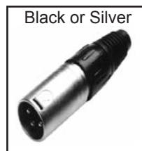
30-529-BK 30-529-SL XLR 3-pin Male plug, twist-on strain relief. .15" to .3" cable opening. Internal compression style cable strain relief.
