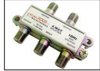
75-712 1GHz 90dB isolation 75-717 1GHz 130dB isolation 4-WAY HIGH ISOLATION SPLITTER 4-way version of 75-710 & 75-715. Specifications 75-712 Insertion Loss 6.8 - 8.2dB 75-717 Insertion Loss 7.0 - 8.2dB Port to port isolation 20 - 25dB Input return loss ..... 15 - 18dB
