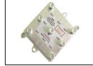
75-713-6 6-WAY 1GHZ DIGITAL SPLITTER 1GHz, 130dB splitter. Digital ready CATV splitters designed for hybrid distribution networks, voice-data, modem and digital converter applications. Fully water resistant. Soldered rear cover 130dB min, EMI-RFI shielding, DC blocked and IEEE-587 built-in 6kV surge protection at all ports. High performance components and circuitry. Anti-corrosion tin plated zinc-alloy, die cast housing. Mounting tabs with screws, cast-in ground block. Insertion loss 9.5-11dB max, isolation 35dB min, isolation 25dB min 40MHz-1GHz. Return loss 22dB min 15-40MHz.
