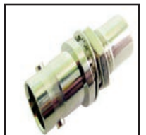
75-521-3/8 Panel feed thru connector. BNC Female to RCA Female. Bushing dia.: .365" Bushing length: .27" Overall length is 1.06" Mounts in .375" hole.
