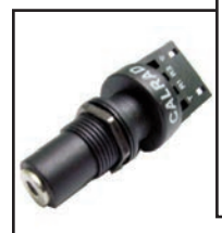
30-712K-S Solderless Keystone & Chassis Mount 3.5mm stereo Jack. 1/2" chassis mount or keystone insert. Screw terminals provide a clean solderless termination. 18 to 30 gauge wire.
