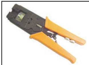
75-599A COMPRESSION CRIMPING TOOL Crimping tool for (CATV) type weather proof compression connectors (RG-59, RG-6, tri/quad shields). Comes with interchangeable dies for RCA, BNC and 'F' Connectors. Dies attach to tool handle for easy storage and access. For use with Calrad 75-533-PS, 75-534-PS, series connectors, including Quad versions
