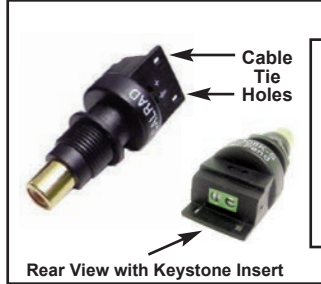
30-308K-S New Solderless Keystone & Chassis Mount RCA Jack. Easily mountable RCA jack for either 1/2" chassis mount or keystone insert. Screw terminals provide for a clean solderless backside termination. For use with 18 to 30 gauge wire. Terminals are marked for easy identification. Includes cable tie for strain relief. Colored plastic washer available for enhanced visual ID.
