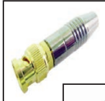
75-800G-75 75 ohm. RG-59 solder BNC connectors, gold with black chrome body. .255" cable opening.
