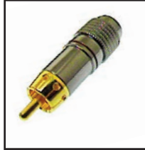
30-302-COLOR Gold plated RCA Audio & Video Plug with teflon insulator for 6-8mm cable. Black chrome barrel with easy grip knurling. .35" cable opening. Available in black, red, white, yellow
