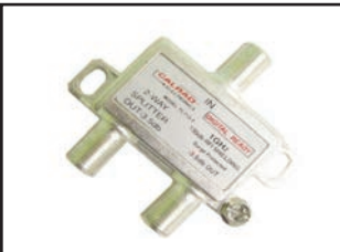
75-713-2 2-WAY 1GHZ DIGITAL SPLITTER 1GHz, 130dB splitter. Digital ready CATV splitters designed for hybrid distribution networks, voice-data, modem and digital converter applications. Fully water resistant. Soldered rear cover 130dB min, EMI-RFI shielding, DC blocked and IEEE-587 built-in 6kV surge protection at all ports. High performance components and circuitry. Anti-corrosion tin plated zinc-alloy, die cast housing. Mounting tabs with screws, cast-in ground block. Insertion loss 3.5-3.7dB max, isolation 35dB min, isolation 30 dB, 15-50 MHz. Return loss 22dB min.
