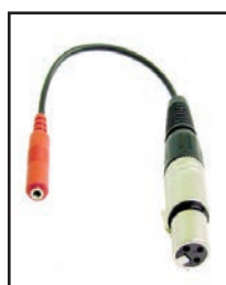
35-467 3.5mm stereo Female jack to XLR Female plug. Wired: pin 1 = ground pin 2 = tip pin 3 = ring. 8" long with Black PVC jacket.
