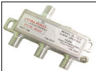
75-713-3 3-WAY 1GHZ DIGITAL SPLITTER 1GHz, 130dB splitter. Digital ready CATV splitters designed for hybrid distribution networks, voice-data, modem and digital converter applications. Fully water resistant. Soldered rear cover 130dB min, EMI-RFI shielding, DC blocked and IEEE-587 built-in 6kV surge protection at all ports. High performance components and circuitry. Anti-corrosion tin plated zinc-alloy, die cast housing. Mounting tabs with screws, cast-in ground block. Insertion loss 3.5-3.7dB max, isolation 35dB min, isolation 21dB min 40MHz-1GHz. Return loss 22db min 15-40MHz.
