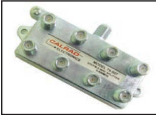
75-507 8-WAY COAXIAL SPLITTER UHF/VHF indoor-outdoor splitter. 75 \Omega . 1 input to 8 outputs. Frequency response of 5 to 900 MHz. Zinc die cast construction with mounting tabs and screws and cast in grounding black. Precision machined threads. Anti-corrosion plating and epoxy sealed.
