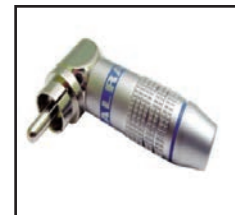
30-250-COLORS Solder type R/A reduced profile RCA style plugs. Polished nickel finish. Available with black, blue, green, orange, red, white, yellow ID bands. For use with 6mm O.D. cable. Solid center conductor. Large 2 finger cable strain relief. Specify color when ordering.
