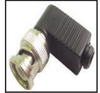
75-559-75 75 ohm version 75-559 50 ohm version Solderless BNC Male right angle connector for use with RG-59 coax cable. Cable opening .24". Black snap style plastic body.
