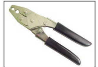
75-560 CRIMPING TOOL Crimping tool for installing F-56, F-59 connectors and others on coax cables. Crimper has 2 openings for various diameter ferrules.
