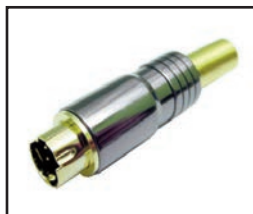
30-505 (4 pin) 30-505-6 (6 pin) 30-505-8 (8 pin) Pro quality Mini Din connector for 5-7mm cable. Metal housing with gold pins, contacts and strain relief. .27" cable opening.
