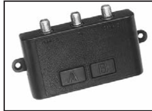
40-695A A/B COAXIAL PUSHBUTTON RF SWITCH High isolation RF A/B pushbutton switch. Complies with FCC part 15.6. 75 ohm RF "F" Female connectors. Lets you select from two inputs. Reversible. 80dB isolation. Frequency 5-900 MHz.
