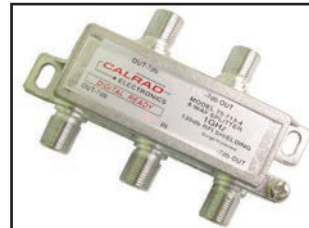
75-713-4 4-WAY 1GHZ DIGITAL SPLITTER 1GHz, 130dB splitter. Digital ready CATV splitters designed for hybrid distribution networks, voice-data, modem and digital converter applications. Fully water resistant. Soldered rear cover 130dB min, EMI-RFI shielding, DC blocked and IEEE-587 built-in 6kV surge protection at all ports. High performance components and circuitry. Anti-corrosion tin plated zinc-alloy, die cast housing. Mounting tabs with screws, cast-in ground block. Insertion loss 3.5-3.7dB max, isolation 35dB min, isolation 21dB min 40MHz-1GHz. Return loss 22dB min 15-40MHz.
