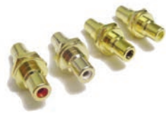
30-410-COLOR NICKEL 30-410G-COLOR GOLD Mounts in 1/2" hole. Bushing length .29" Overall length 1.3"
