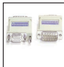
30-594 10 position 30-593 6 position VGA to MAC adapter, 10 position or 6 position Dip Switch For connecting Apple DB15 pin to HDDB15 pin. Supports Apple standard display modes. Dip switches select different display modes.
