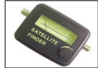
75-728 Analog Meter 75-729 Digital Meter SATELLITE FINDER METERS Highly sensitive meters. 75ohm, frequency range 950-2050MHz input. Sensitivity 7mV @ 55dB, LNB Gain 3-Carrier C/N 15dB, Input level -25dBm to -75 dBm, LNB gain 52-60dB, power requirement 13-18Vdc from existing coax feed. Requires 6dB attenuator for 60-65dB LNB. 75-728 has a built-in buzzer
