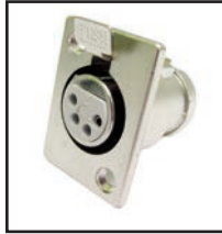
30-523-SL-4 4 pin Silver 30-523-BK-4 4 Pin Black 30-523-SL-5 5 pin Silver 4 or 5 pin Female XLR chassis jack mounts in \frac{15}{16} " hole size.
