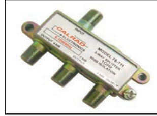
75-711 1GHz 90dB isolation 75-716 1GHz 130dB isolation 3-WAY HIGH ISOLATION SPLITTER 3-way version of 75-710 & 75-715. Specifications 1 Port Insertion Loss 3.5 - 4.5dB 2 Port Insertion Loss 6.8 - 8.2dB Port to port isolation 20 - 25dB Input return loss ..... 15 - 18dB
