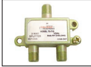
75-710 1GHz 90dB isolation 75-715 1GHz 130dB isolation 2-WAY HIGH ISOLATION SPLITTER 5-1000MHz, 75ohm splitters with precision F connector threads, anti-corrosion zinc die cast case and mounting tabs with screws. Specifications Insertion Loss ..... 3.4 - 4dB Port to port isolation..... 21 - 24dB Input return loss..... 15 - 20dB
