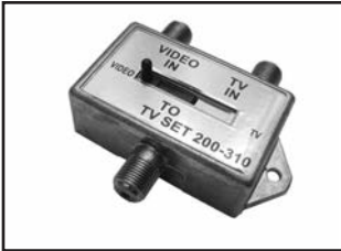
75-496 A+B TV ANTENNA VCR & CABLE SWITCH 75 ohm inputs/output for hook-up of outdoor TV antenna or MATV outlet cable TV or VCR to TV set. 40dB isolation.
