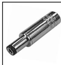
30-363 3.5 mm mini-jack to DC power plug. 3.0 mm coax plug I.D.
