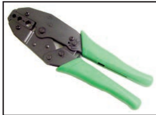
75-569 FULL CYCLE RATCHET CRIMPING TOOL Full-cycle ratchet crimping tool for F, BNC, TNC Connectors RG-58, RG-59, RG-62, Rg-6 & PIN. Jaw Sizes: .0213", .256", .324", PIN = .068".
