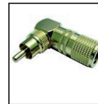
30-305 L=.95" Short Version Right angle RCA Audio & Video plug with heavy gold plating, teflon insulator, for 8mm cable, short version. 30-306 L=1.3" Long Version. .37" cable opening
