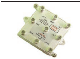
75-713-8 8-WAY 1GHZ DIGITAL SPLITTER 1GHz, 130dB splitter. Digital ready CATV splitters designed for hybrid distribution networks, voice-data, modem and digital converter applications. Fully water resistant. Soldered rear cover 130dB min, EMI-RFI shielding, DC blocked and IEEE-587 built-in 6kV surge protection at all ports. High performance components and circuitry. Anti-corrosion tin plated zinc-alloy, die cast housing. Mounting tabs with screws, cast-in ground block. Insertion loss 9.5-11dB max, isolation 35dB min, isolation 25dB min 40MHz-1GHz. Return loss 22dB min 15-40MHz.
