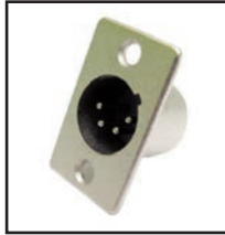
30-522-SL-4 4 Pin 30-522-SL-5 5 Pin 4 or 5 pin Silver Male XLR chassis plug mounts in .75" hole size.
