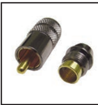
30-354-RG59 30-354-RG6 75 ohm gold RCA Video Connector. Recessed barrel provides a low profile when inserted into a Female jack. Solder center pin at base of connector, fold shield over PVC, a 2 piece twist type compression fitting is used to secure the shield to the connector. Available for RG-59 and RG-6.
