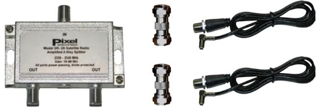
This signal splitter allows the connection of two satellite radios to a single antenna. It has internal diodes that pass DC voltage (antenna 5 VDC power) with less than 0.5 VDC of loss from the radio to the splitter's input port to provide power to the antenna from any radio connected to the outputs. Because of its' internal amplifier (with more than 10 dB net gain), the loss of the splitter is overcome and up to 90 feet of RG-6 cable can be attached to any radio output port.
