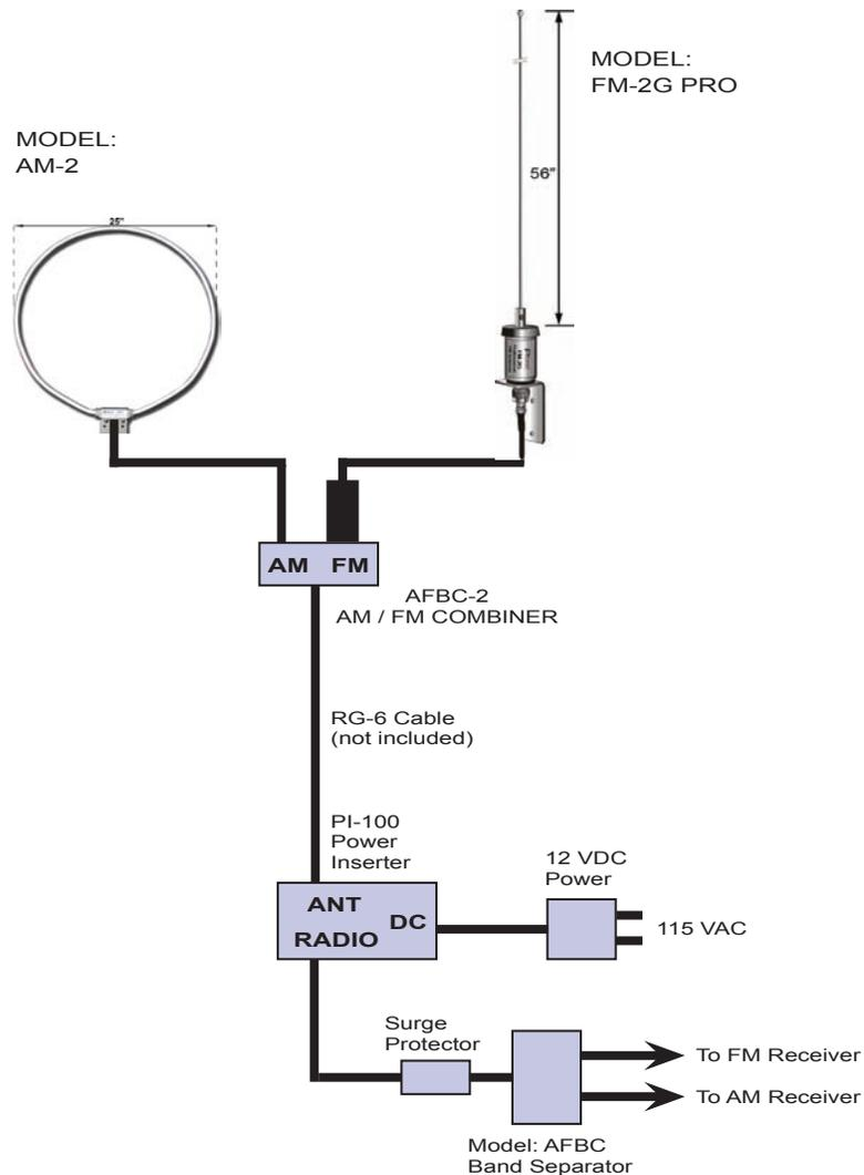
This kit includes everything required for achieving very high quality AM / FM reception. It features the highly-regarded AM-2 Magnetic Loop AM Antenna and the FM-2G PRO Omni-Directional FM base-loaded Dipole. Also included are all the necessary accessories to combine the signals from each antenna on a single lead-in wire and separate them at the AM /FM receiver.
