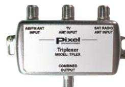
Combines the output of an AM / FM antenna, satellite radio antenna, and television antenna (for channels 7 and higher) onto a single coax cable. Contains a 9 dB satellite radio amplifier. Requires 5 VDC on the coax cable to power the amplifier. Recommended for use with Pixel satellite radio and AM / FM antennas
