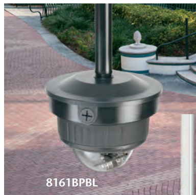
Mounts up to 50 lbs, on a down rod Includes installed threaded base plate and 3/4" to 1/2" reducing bushing for use with 1/2" or 3/4" NPT down rods. (Support pipe not included)
