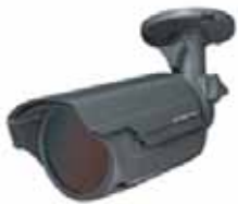
LPRS Series (Illum) License Plate Recognition Camera Captures plates at speeds of up to 30MPH Capture Range up to 60 feet No motion blur 24VDC/AC
