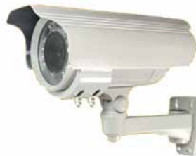
TV-B110 (Tane) Outdoor series 420 TVL 4 – 9 mm 24 IR LEDs 30 ft 12VDC / IP65
