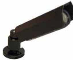
6305-B (Channel-Vision) Color Bullet 330 lines 0.5 lux, F2.0 3.6mm lens Sunshield Included
