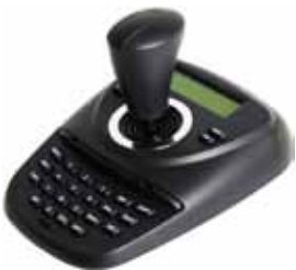
PTZ-3X-CON (Ascendnet) 3-Axis PTZ Controller Pelco D protocol
