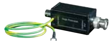
CSP1 (ARM) Coaxial Surge Protection 100ns surge protect attack time 5amp max. surge current Surge life 300 surges
